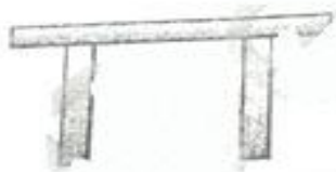
LINTEL BEAM Method (Traditional Indian Method)
