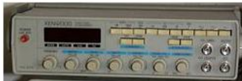
A simple analog function generator, circa 1990
