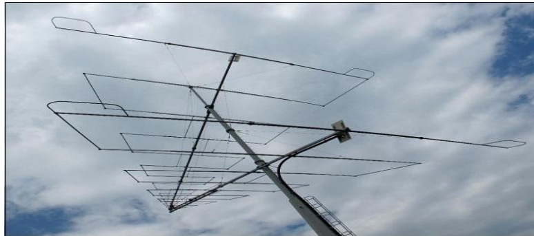
The image shows a log-periodic antenna.
