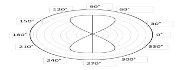
The above figure shows the radiation pattern for normal mode of radiation in helical antenna.
