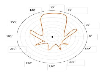
The figure shows the radiation pattern for axial mode of radiation in helical antenna.
