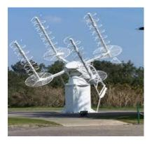
**Helical antenna** or helix antenna is the antenna in which the conducting wire is wound in helical shape and connected to the ground plate with a feeder line. It is the simplest antenna, which provides **circularly polarized waves**. It is used in extra-terrestrial communications in which satellite relays etc., are involved.
