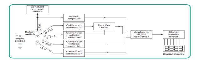
**Block Diagram of Digital Multimeter**
